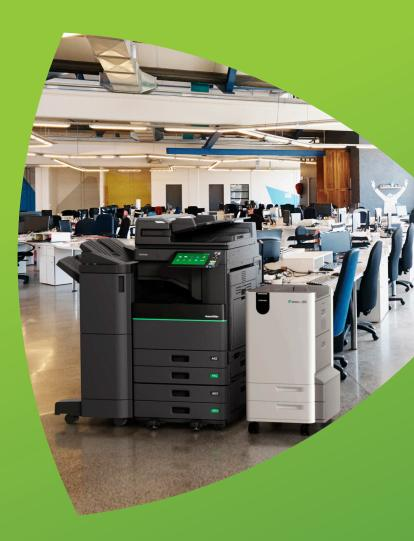
The Paper Reusing Device (PRD) is an option for the e-STUDIO5008LP series which uses erasable blue toner. It not only erases paper, the device is also capable of scanning documents for archiving and document retrieval. Equipped with a single pass duplex scanner the system ensures fast conversion into JPEG, TIFF or PDF format. These files are then stored on your server and become part of your digital archive. Providing access to your content whenever you need it.
